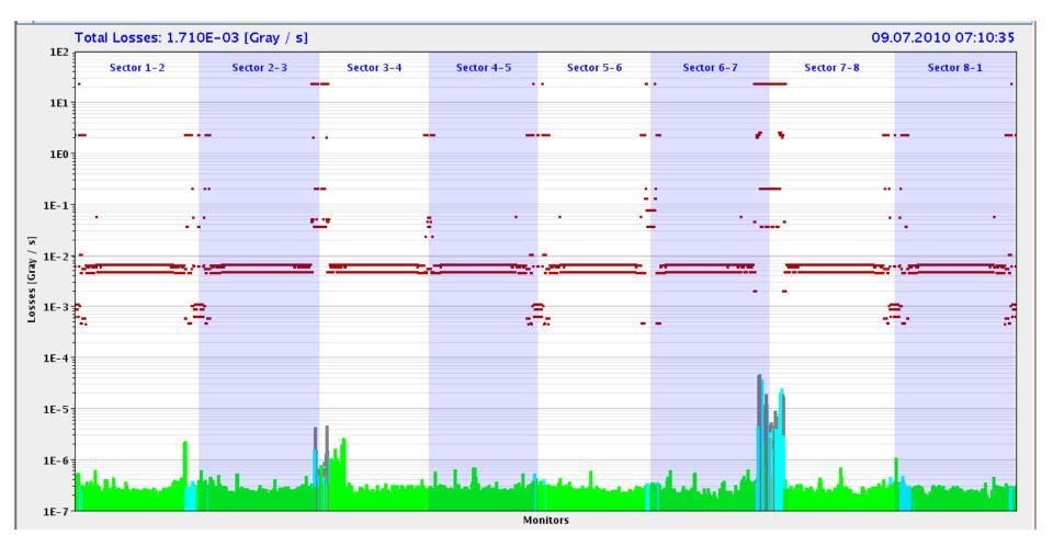
Takes place at collimators in cleaning insertions → OK
