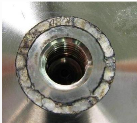
Contact erosion series diode stack not sufficiently tightened
