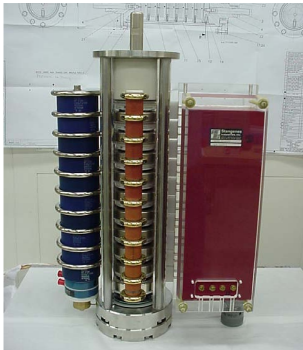
Figure 1: One of two HV switches of an MKD generator: GTO stack (centre), partly hidden behind the voltage distribution resistors; trigger transformer (right); snubber capacitors (left).
