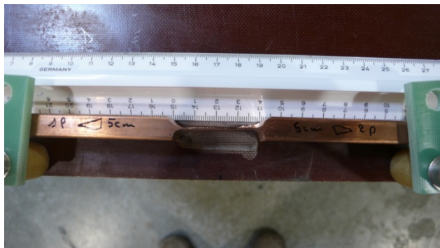
Figure 6: A picture of the defect machined out of a solid copper bar for the Thermal Amplifier tests in Block 4. This represents a defect of about 50uOhms at room temperature.
