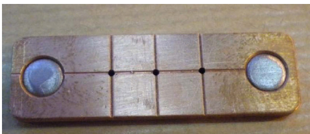
Figure 3. Shunt prototype integrating solder alloy reservoir, capillarity grooves and degassing holes
