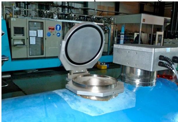
Figure 1: Self closing over pressure valve
