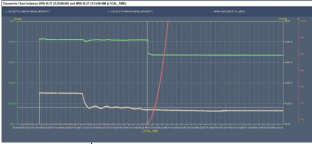
Figure 6: Oct 27 th , fill 1450, 150 ns spacing, 368 bunches, 4.3E13 p total per beam. Beam 1 Fast BCT (beige), DC BCT (green) at beginning of ramp (red). The loss corresponds to 1.6E12 p.
