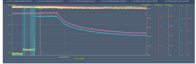
Figure 3: Single bunch nominal intensity. Fast BCT and four-sigma bunch length through the ramp. The bunch shrinks from 1.5-1.7 ns on the flat bottom to 0.8-0.9 ns at 3.5 TeV.
