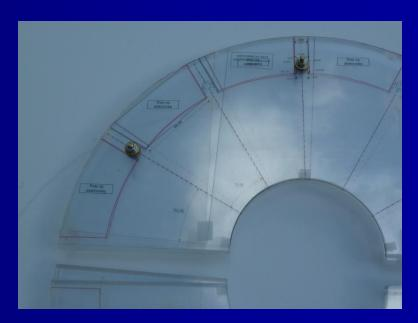
Simple model in 1:1 scale of a part of the mechanical structure from transparent plastics has been made to proof the design.
