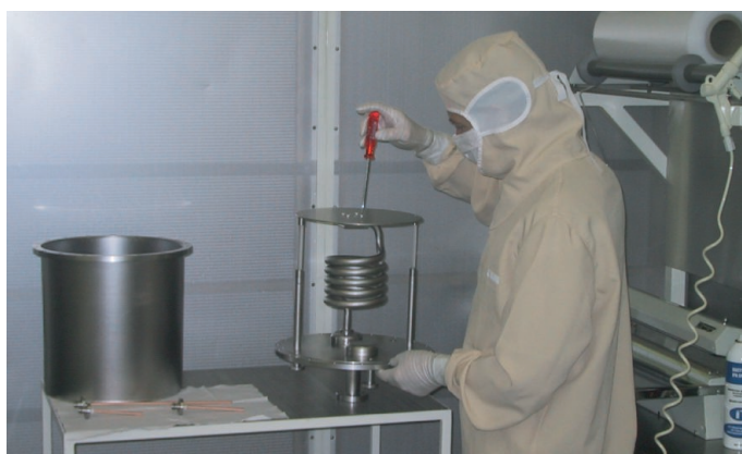
Figure 3.1: Cryogenic superconducting niobium test cavity being cleaned by water jet and assembled in a clean room at CERN.
