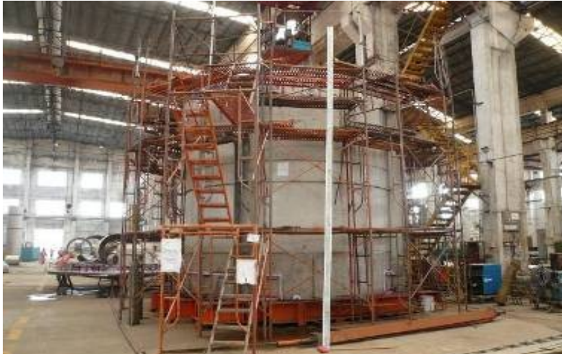
SSV under fabrication, tests include full load, negative pressure, laser survey, etc.
