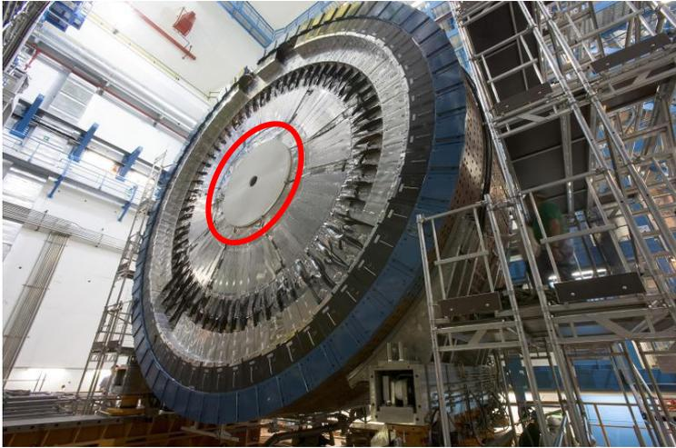
MinBias Trigger Scintillator at  $z=\pm 3.56$  m
