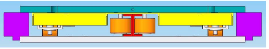
Platform raised by hydraulic jacks by 9mm. Guide Rail and Rollers prevent module from toppling (high centre of gravity).
