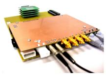
A full mechanical model of DBB and FEB was produced in order to test the assembly and accessibility of different connectors.
