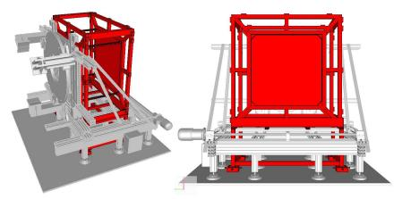
The bottom chassis and related x-y-z system (x4) to tune the EMR position with respect to KL are under development.
