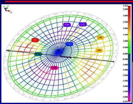
Plot of the laser inspection machine data Distorted window
