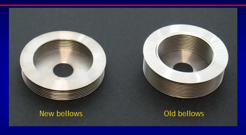
Sample bellows from a new vendor is at LBNL for testing
