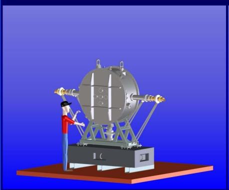
MTA beam height configuration on concrete block
