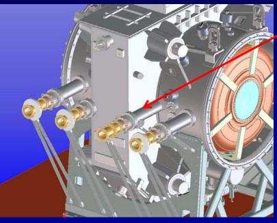
Scallop in coupling coil cryostat for the RF coupler
