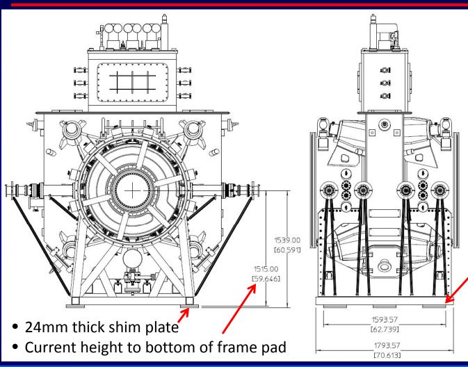
RFCC module frame mounting plates moved inboard by 100mm
