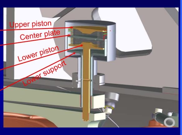
• Actuator mechanical components (except bellows) for 6 actuators are being fabricated at University of Mississippi (D. Summers and M. Reep)
