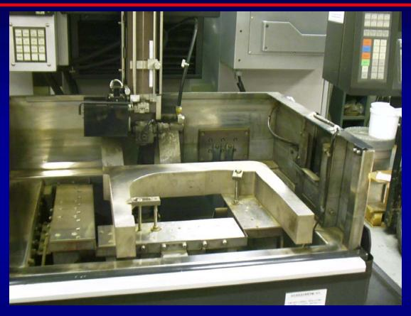
• Six tuner flexures are being fabricated at the University of Mississippi (D. Summers and M. Reep)
