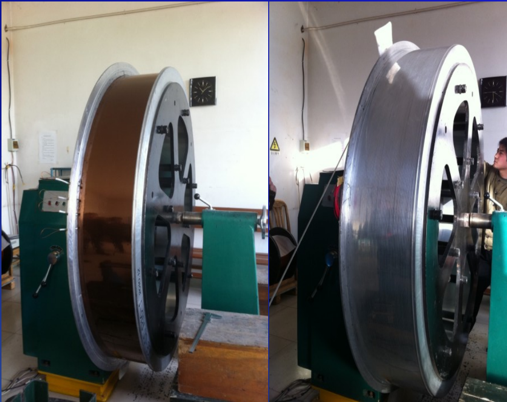
Coil winding at Qi Huan: last layer of SC wire (left) and finished Al banding (right)
