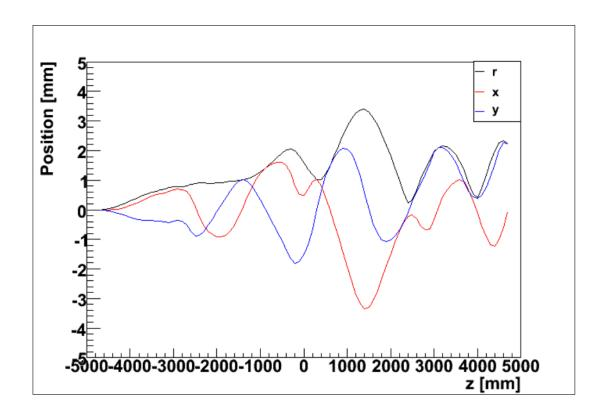
Displacement of reference muon due to shield error fields
