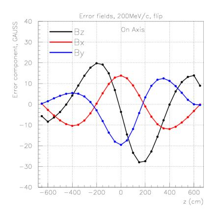
$B_x \sim 12 \sin (2 \pi x / 7 \text{ metres}) \text{ Gauss}$
