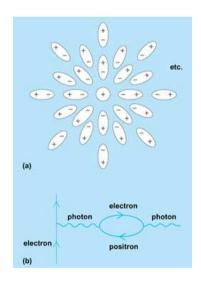
The strong coupling  $\alpha_3$  is anti-screened due to gluon self-interactions
