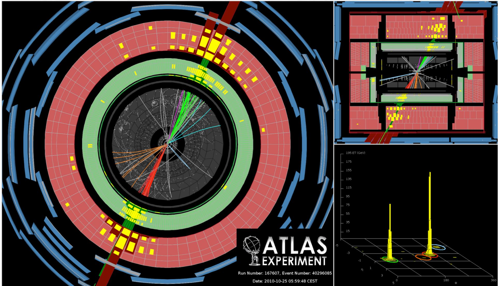
Event display that shows the highest-mass central dijet event collected during 2010, where the two leading jets have an invariant mass of 3.1 TeV. The two leading jets have  $(p_T, y)$  of (1.3 TeV, -0.68) and (1.2 TeV, 0.64), respectively. The missing  $E_T$  in the event is 46 GeV. From [ATLAS-CONF-2011-047](#).
