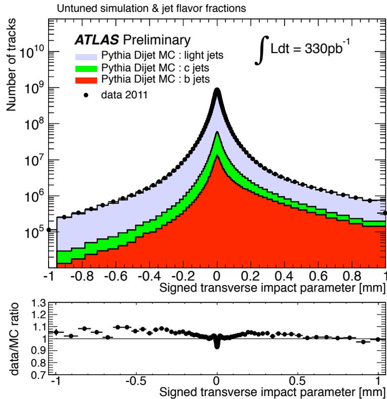
Distribution of the signed transverse impact parameter with respect to primary vertex for tracks of b-tagging quality associated to jets, for experimental data (solid black points) and for simulated data (filled histograms for the various flavors). The ratio data/simulation is shown at the bottom of the plot.
