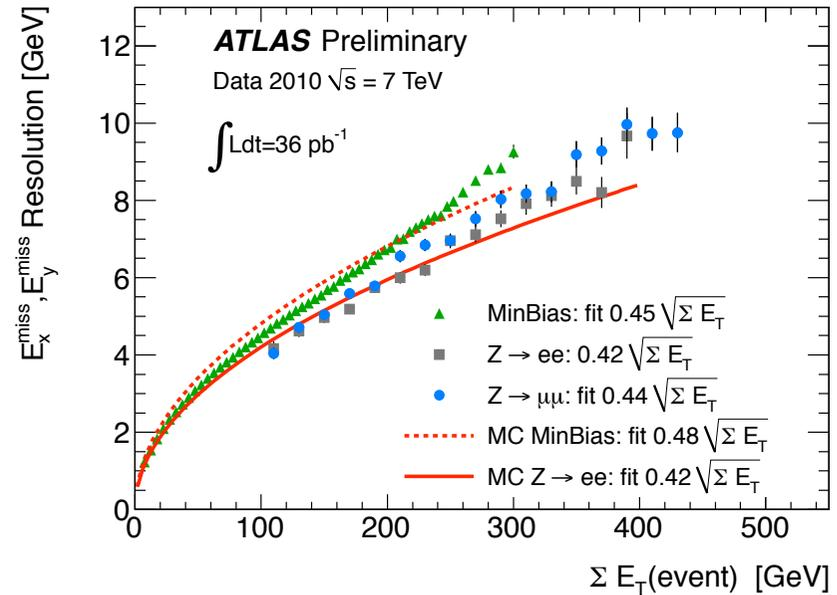
Resolution of  $E_x^{\text{miss}}$  and  $E_y^{\text{miss}}$  as a function of the total transverse energy in the event calculated by summing the  $p_T$  of muons and the total calorimeter energy. The resolution in  $Z \rightarrow ee$  and  $Z \rightarrow \mu\mu$  events is compared with the resolution in minimum bias for data taken at  $\sqrt{s} = 7$  TeV. The fit to the resolution in Monte Carlo minimum bias and  $Z \rightarrow ee$  events are superposed.
