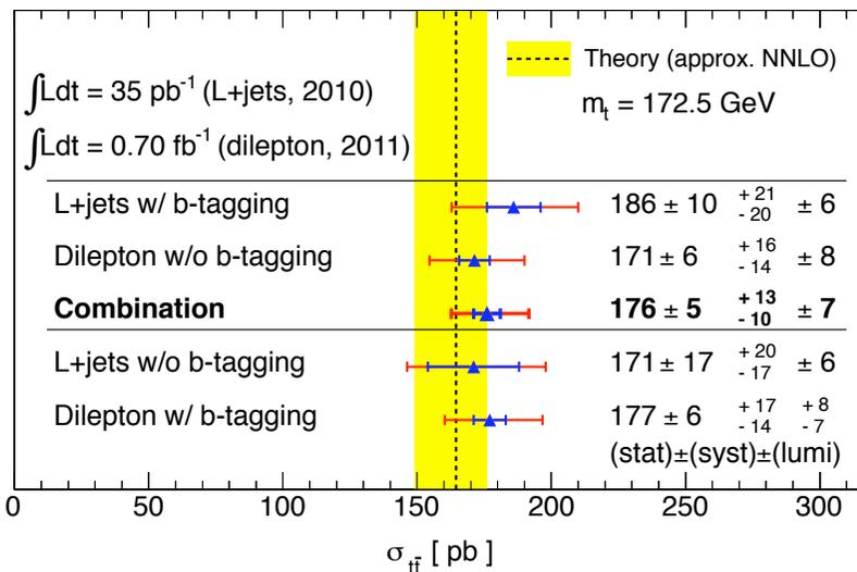
Best fit (ATLAS) gives a slightly higher cross-section than the expected approx. NNLO QCD value, but consistent within  $1 \sigma$  (red: likelihood, stat errors only; blue: stat + syst. uncertainties)
