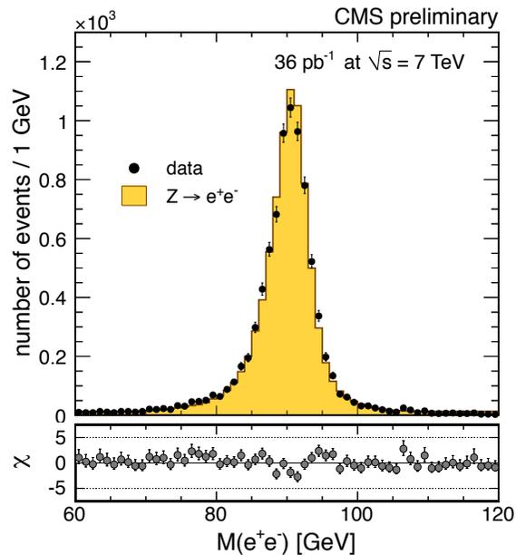
Distributions of the invariant di-electron mass,  $m_{ee}$ , for events passing the Z selection. The data are compared to Monte-Carlo simulation, the background is very small.
