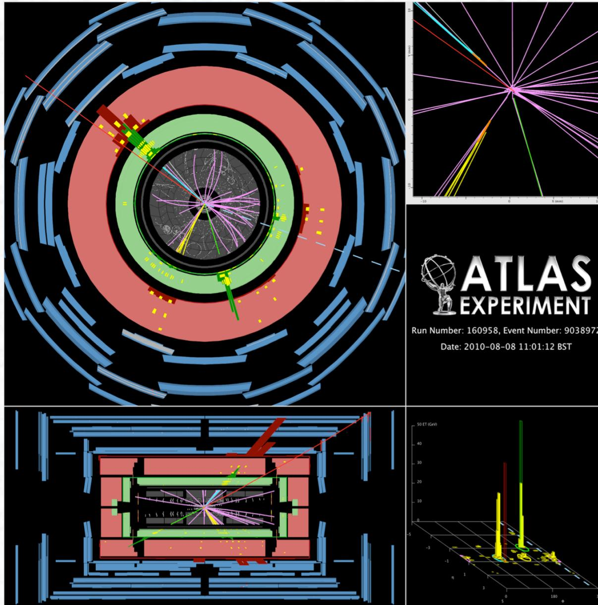
Event display of a top pair  $e\text{-}\mu$  dilepton candidate with two b-tagged jets. The electron is shown by the green track pointing to a calorimeter cluster, the muon by the long red track intersecting the muon chambers, and the missing  $E_T$  direction by the dotted line on the xy-view. The secondary vertices of the two b-tagged jets are indicated by the orange ellipses on the zoomed vertex region view.
