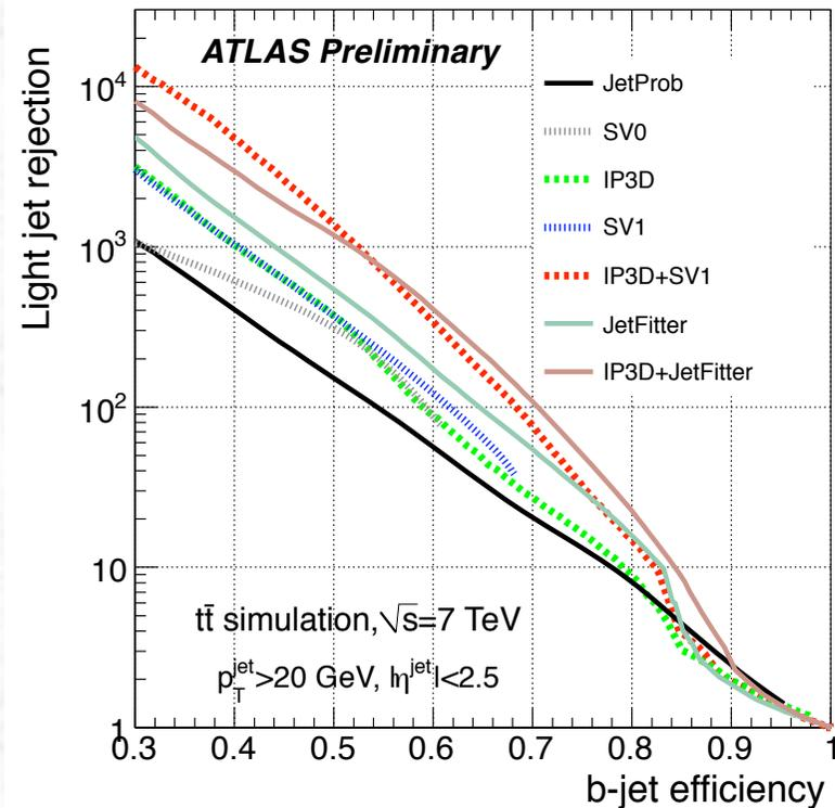
Light-jet rejection as a function of the b-jet tagging efficiency for the early tagging algorithms (JetProb and SV0) and for the high performance algorithms, based on simulated top-antitop events.
