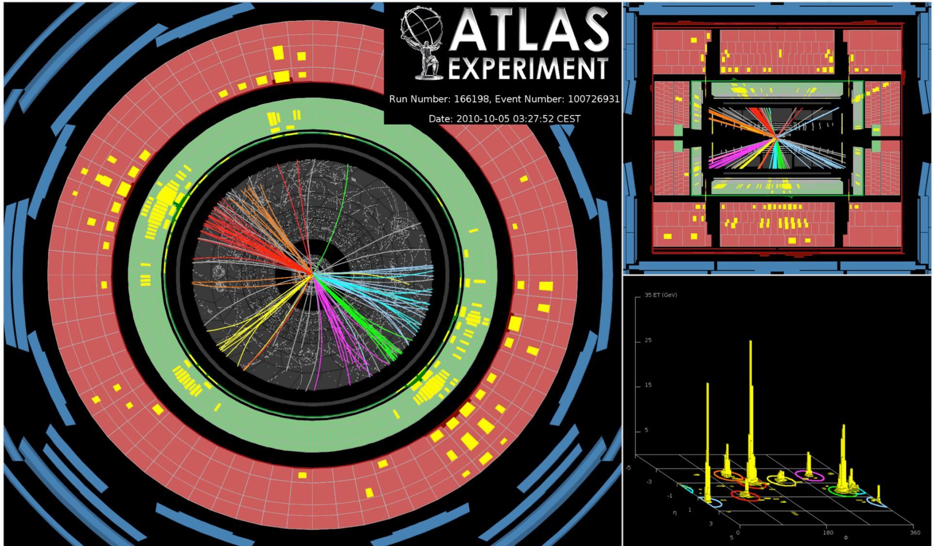
The highest jet multiplicity event collected, counting jets with  $p_T$  greater than 60 GeV: this event has eight. 1st jet (ordered by  $p_T$ ):  $p_T = 290$  GeV,  $\eta = -0.9$ ,  $\phi = 2.7$ ; 2nd jet:  $p_T = 220$  GeV,  $\eta = 0.3$ ,  $\phi = -0.7$  Missing  $E_T = 21$  GeV,  $\phi = -1.9$ , Sum  $E_T = 890$  GeV.
