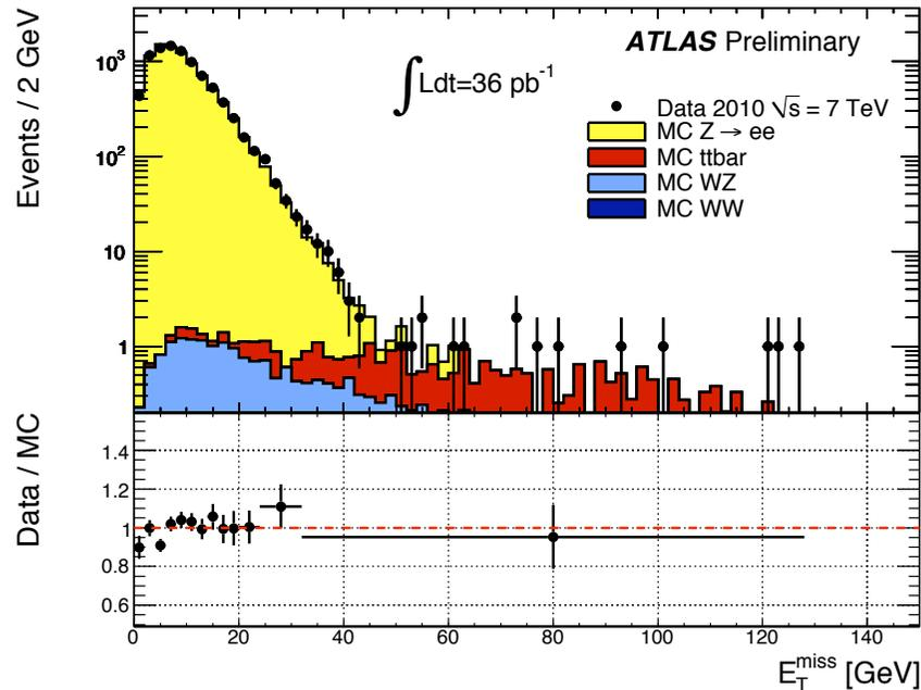
Distribution of  $E_T^{\text{miss}}$  as measured in a data sample of  $Z \rightarrow ee$  events. The expectation from Monte Carlo simulation is superimposed (histogram) and normalized to data, after each Monte Carlo sample is weighted with its corresponding cross-section. The ratio of the data distribution and the Monte Carlo distribution is shown below the plot.
