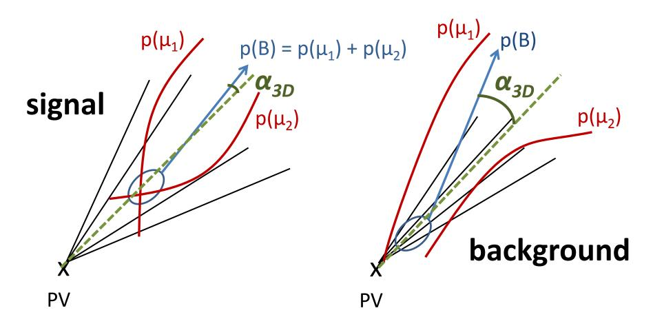
Angle between p(B) and vector between PV and dimuon vertex
