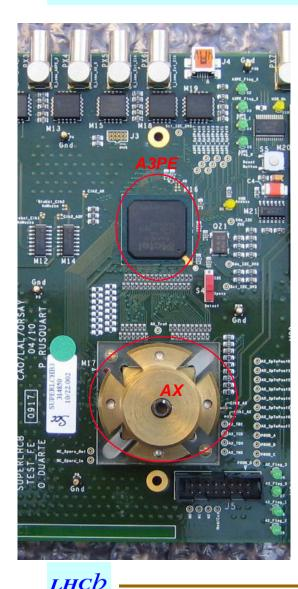
Idea : RAM pattern to test the A3PE IOs functioning by exchanging data between the 2 FPGA (SSO and SSI)
