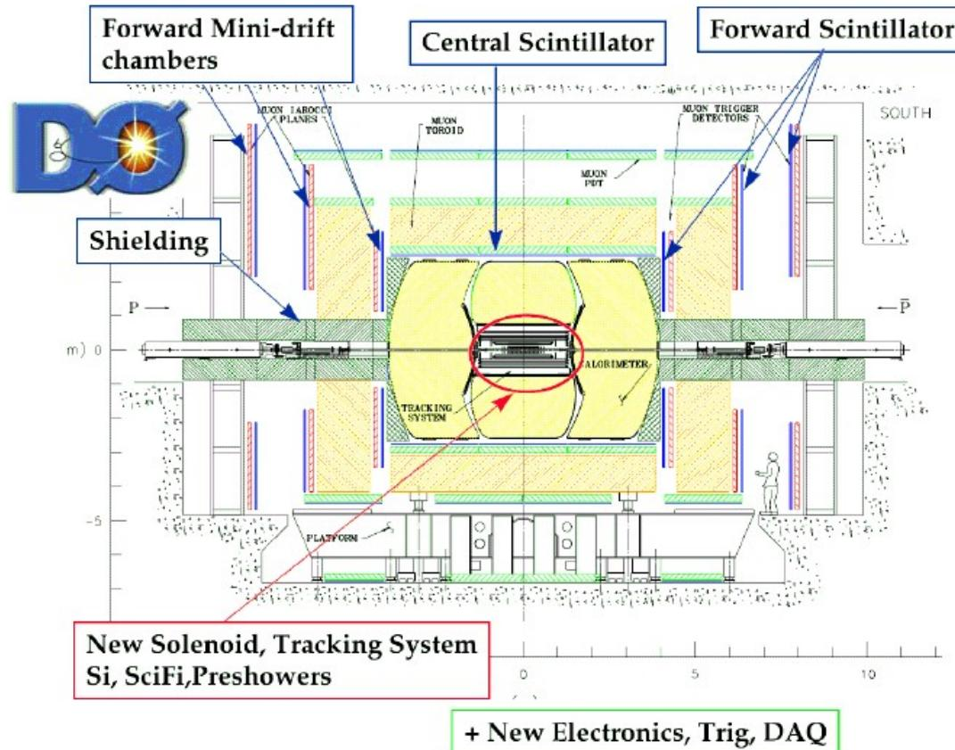
Multipurpose detectors able to reconstruct (and identify)  $e$ ,  $\mu$ ,  $\tau$ , light and heavy jets, missing transverse energy  $E_T$
