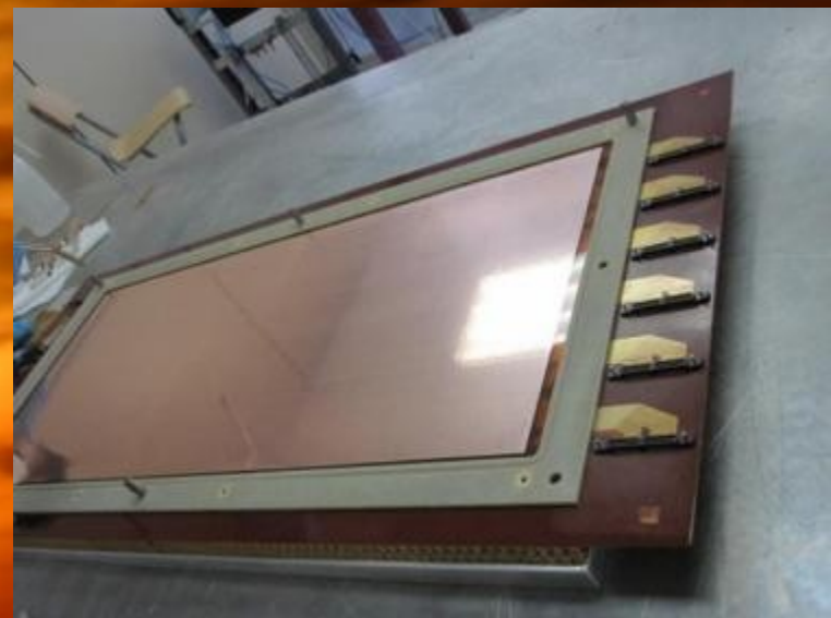
first GEM framed and placed on the readout
