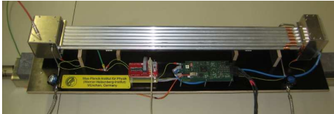
Figure 7: Photograph of the drift tube chamber and part of the read-out electronics.
