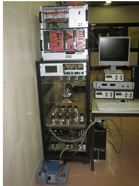
Figure 8: Photograph of the gas system used to mix the Ar/CO 2 drift gas. On the top the NIM and VME crates containing the trigger logic and read-out modules are visible, on the right side the low voltage and high voltage power supplies for the drift tube chamber and the trigger scintillators.
