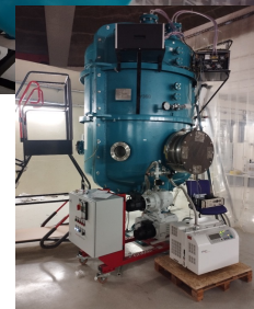
Checking HV vessel tightness (Sept 22)
