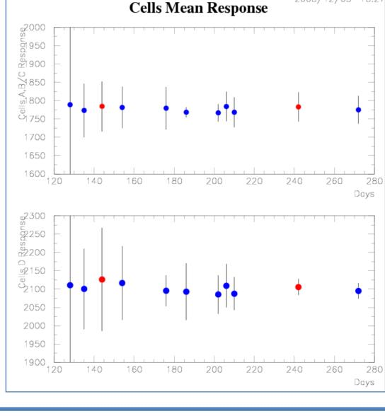
Preliminary estimations of cell mean responses showed good stability around 0.3% by the end of 2008 year. Initial big RMS is reduced after the end of equalization period in the middle of the year. Further efforts to improve the results are under way
