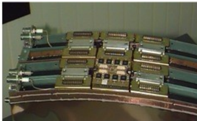
End-Cap Wheel prototype: Front-End Electronics connections
