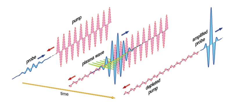
•A long laser pulse (pump) in plasma will spontaneously scatter off Langmuir waves: Raman scattering Stimulate this scattering by sending in a short, counter propagating pulse at the frequency of the scattered light (probe pulse) Because scattering happens mainly at the location of the probe, most of the energy of the long pump will go into the short probe: efficient pulse compression
