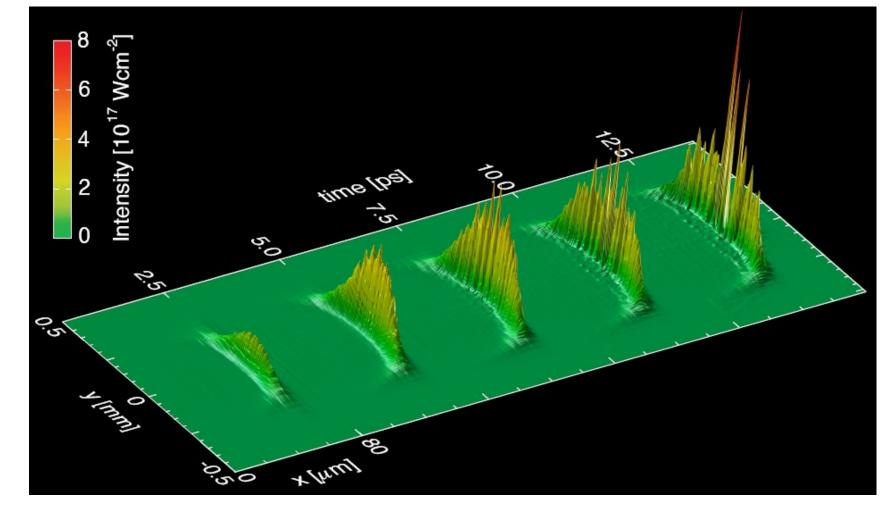
For a 2\*10<sup>15</sup> W/cm<sup>2</sup> pump and  $\omega_0/\omega_p$  = 10, the probe is still amplified, but also destroyed by filamentation
