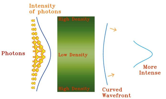
Physical mechanism for self-focusing driven by the ponderomotive force, relativistic mass increase or thermal effects.
