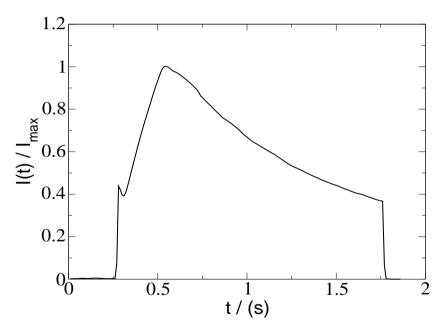
After sufficiently long time transverse beam shape and time evolution of beam current become independent of initial beam shape.
