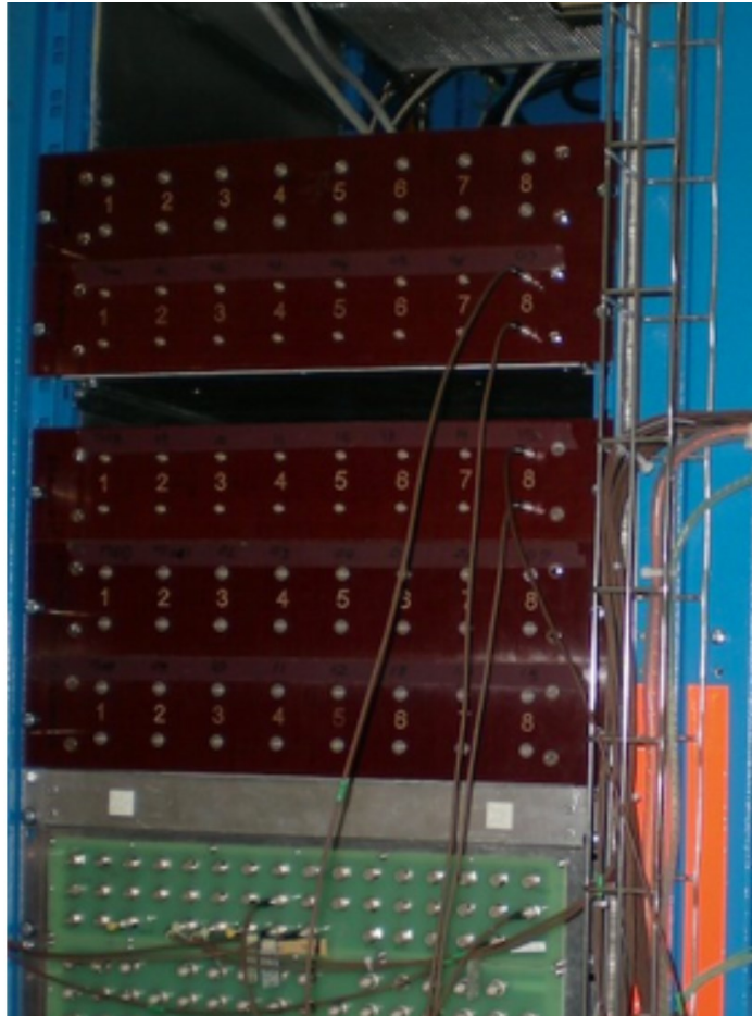
60 m long coax cable per delay line
