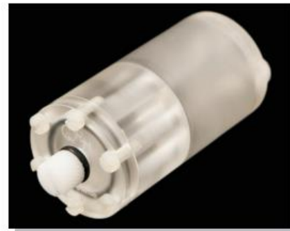
Micro-PET IQ Phantom (according to NEMA NU 4-2008)
