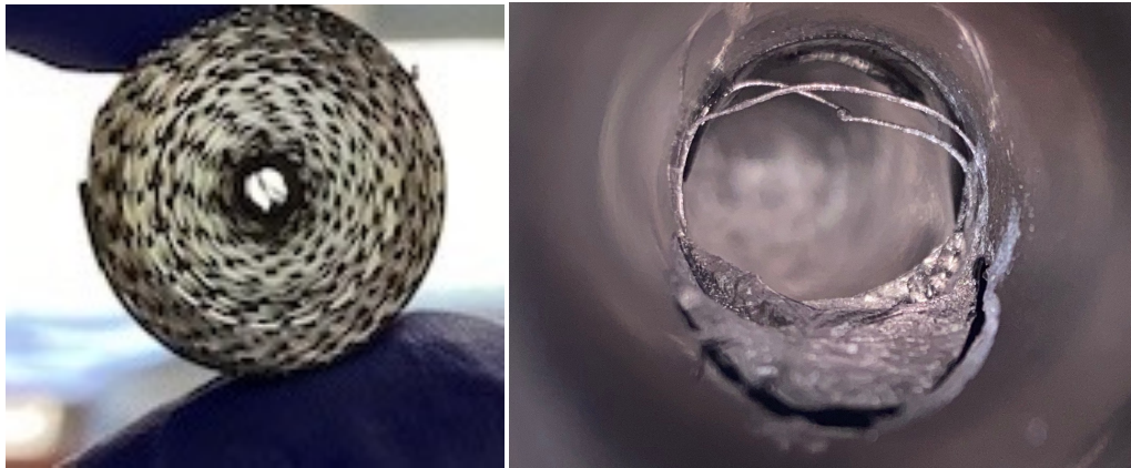
Intact (left) and molten (right) Ti roll target material.
