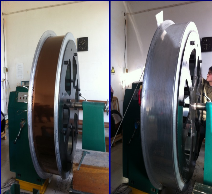
Coil winding at Qi Huan: last layer of SC wire (left) and finished Al banding (right)
