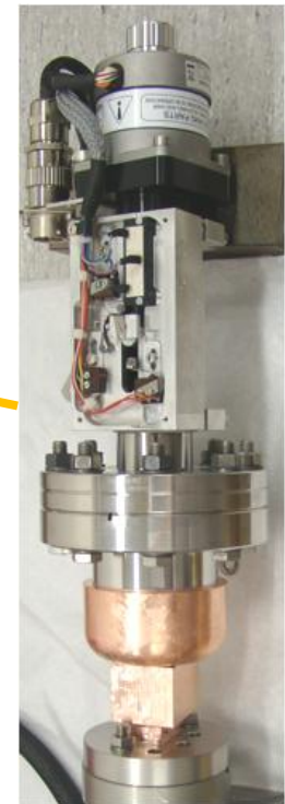
Movable RF short circuit (for tuning the resonant length)
