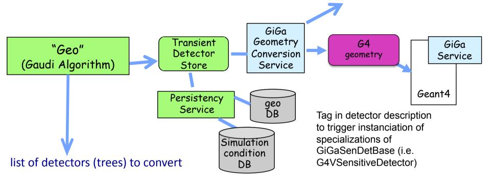
The list controllable for default LHCb detector via a simple Gauss configuration Can give different list: switch off some detectors, add some new, test beam or upgrade
