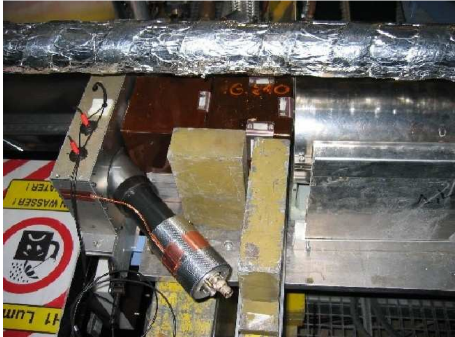
Figure 5: The compact water Cherenkov counter in the operating position in the tunnel of the HERA collider. The left relative to the beam arm of the counter with entering it PM is seen.
