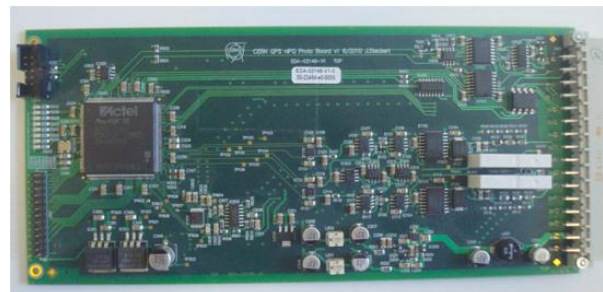
Figure 7: Radiation tolerant FPGA based quench detection board for the protection of insertion region magnets.
