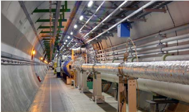
"Combined" sector both side of each experiment Both beams circulates in the same beam pipe
