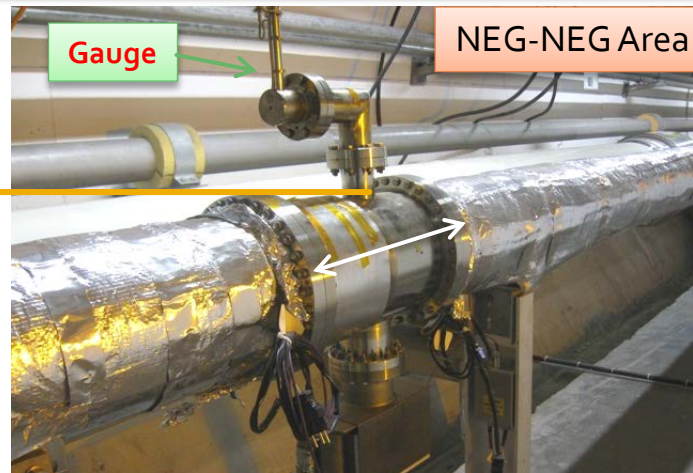
Uncoated parts in the room temperature beam pipes
