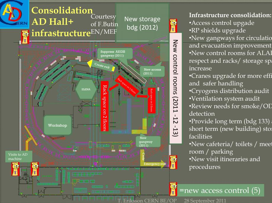
•Access control upgade •RP shields upgrade •New gangways for circulation and evacuation improvement •New control rooms for ALARA respect and racks/ storage space increase •Cranes upgrade for more efficient and safer handling •Cryogens distribution audit •Ventilation system audit •Review needs for smoke/ODH detection •Provide long term (bdg 133) and short term (new building) storage
