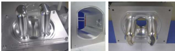
Figure 22: Pictures of the first Aluminum prototype cavity of the 4-rod structure.
