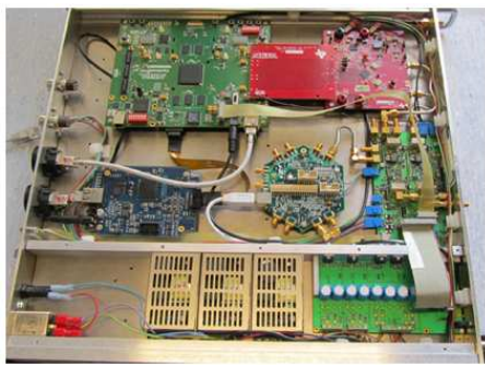
Figure 5: Prototype installation of beam current change monitor
