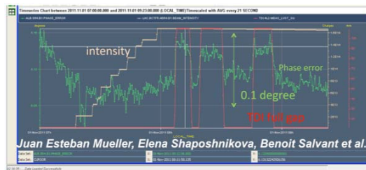
Figure 21: TDI power loss estimated by measuring the synchronous phase shift as a function of the distance between the two jaws.
