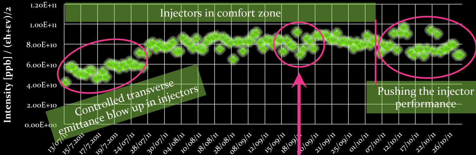
LHC 50 ns bunch intensity out of SPS 13/07/2011 - 30/10/2011
