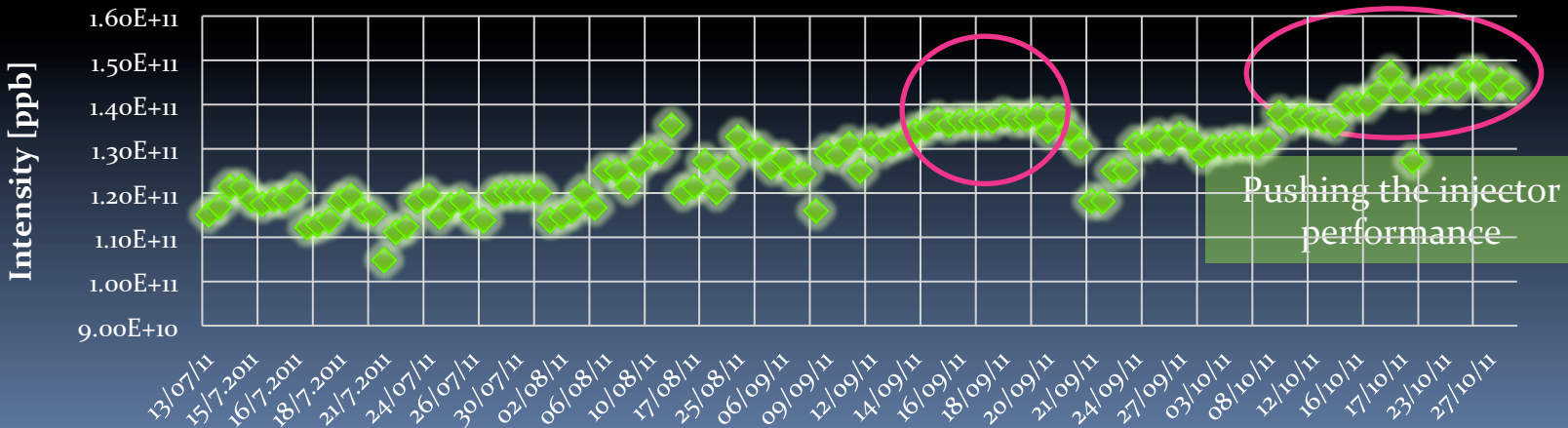
LHC 50 ns bunch intensity out of SPS 13/07/2011 - 30/10/2011
