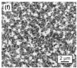
Nanostructure can melt even at 0.1 MJm<sup>-2</sup> because the thermal diffusivity significantly decreased. (Kajita, NF(2007))
