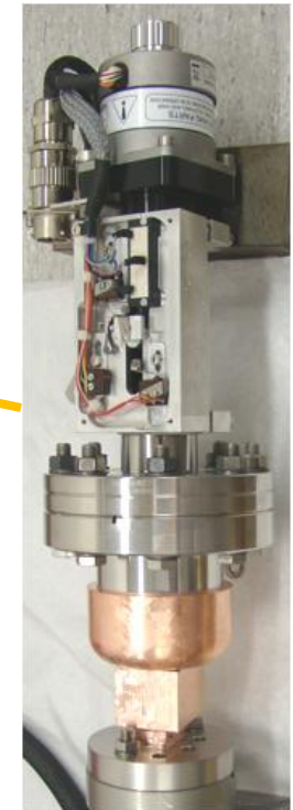
Movable RF short circuit (to tune the resonant length)
