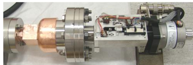
In CTF3 a movable short is added, to allow for recirculation mode
