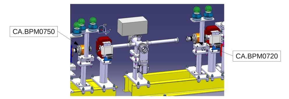
These BPMs are likely to be immune to the low-freq (<100 MHz) noise induced by the drive beam on the diagnostics  $\rightarrow$  back-up solution for the kick measurement
