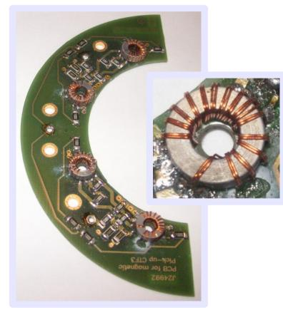
• 40 new toroids (8 toroids per BPM x 5 BPMs) with 10 turns each (currently 30) are being produced at Uppsala and will be assembled at CERN on the existing PCBs
