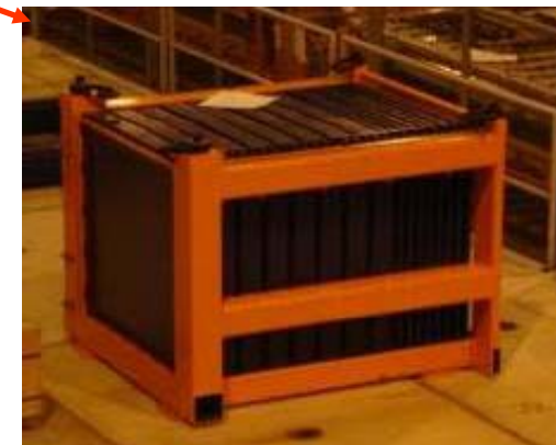
Scint. Strips-Fe Tail Catcher & Muon Tracker 5x100cm 2 strips ~5 λ in 16 layer
