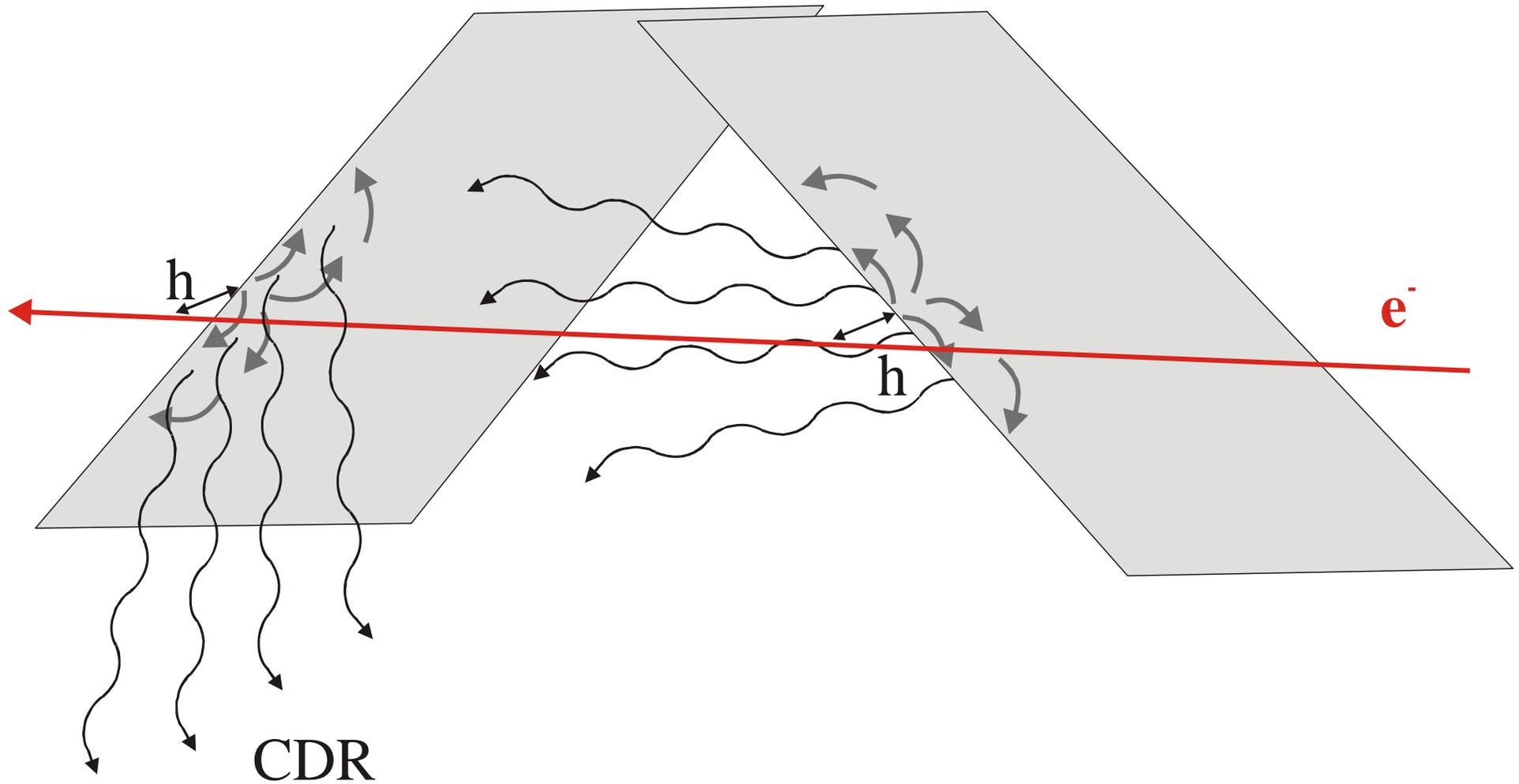
**An electron beam passes by two screens with  $h$  being the impact parameter. Advantage is that much less exclusive beam time is required.**
