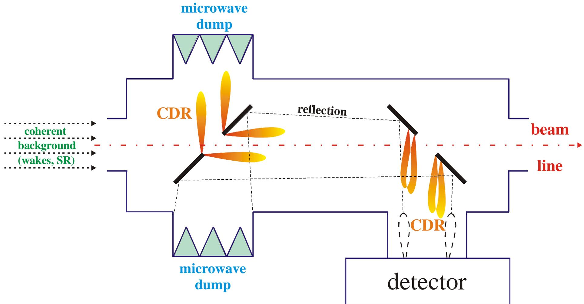
As a detector module one might use an interferometer system for the beginning to be able to develop the bunch diagnostics method. A single shot grating type spectrometer system is also considered.
