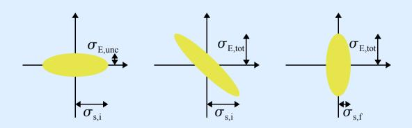
$$\sigma_{\text{s,f}} = \sqrt{\left(1 - \frac{1}{E_0} \frac{dE}{ds} R_{56}\right) \sigma_{s,i}^2 + R_{56}^2 \left(\frac{\sigma_{\text{E,unc}}}{E_0}\right)^2}$$
