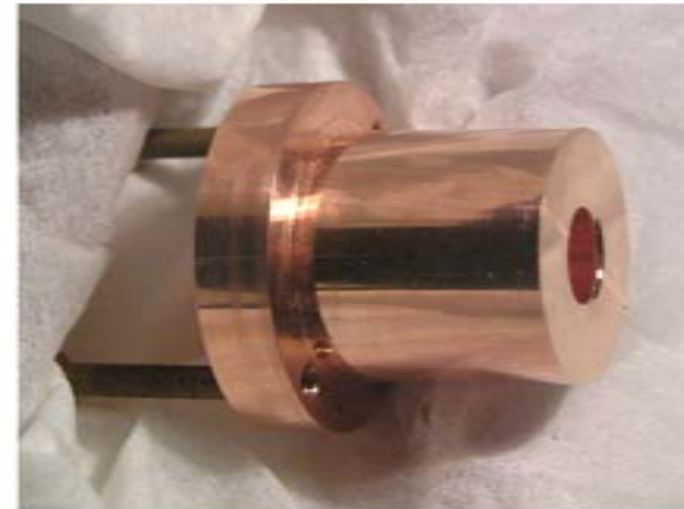
Details of test cavity – vacuum box, central ring and input diaphragm
