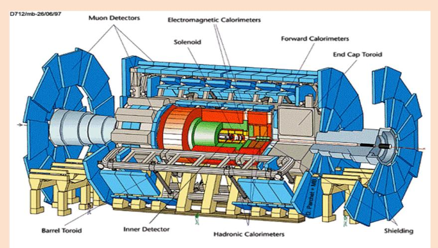
FIG. 1: Lay-out of the ATLAS detector with its major sub-system components. The diameter is about 25m, the total length about 46m, and the weight 7000 Tons.
