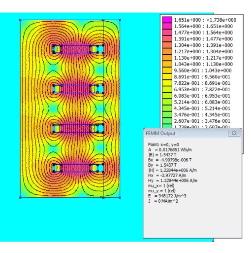
2D Study of 0.44 m reduction for the external dump scenario, 1.55 T at 2 GeV, maximum limit!
