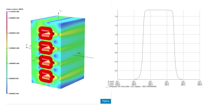
Basic 3D study- shows approximately 1.2 % reduction in integrated field due to the heavily saturated pole ends.
